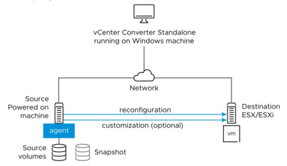
5. Optionally, Converter Standalone uninstalls the agent from the source machine. The virtual machine is ready to run on the destination server.
