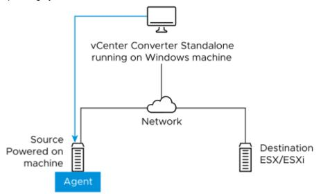
2. Converter Standalone creates a virtual machine on the destination machine.
