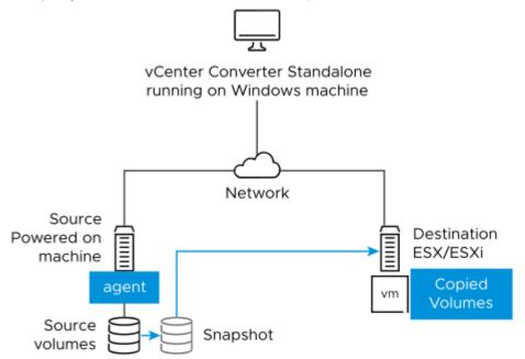
If the proxy mode feature is on, the data traffic passes from the source machine through the Converter Standalone server to the destination server.
