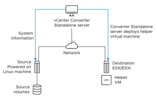
2. The helper virtual machine powers on, boots from the Linux image, connects to the source machine through SSH, and starts retrieving the selected data from the source. While you set up the conversion task, you can select which source volumes to be copied to the destination machine.
